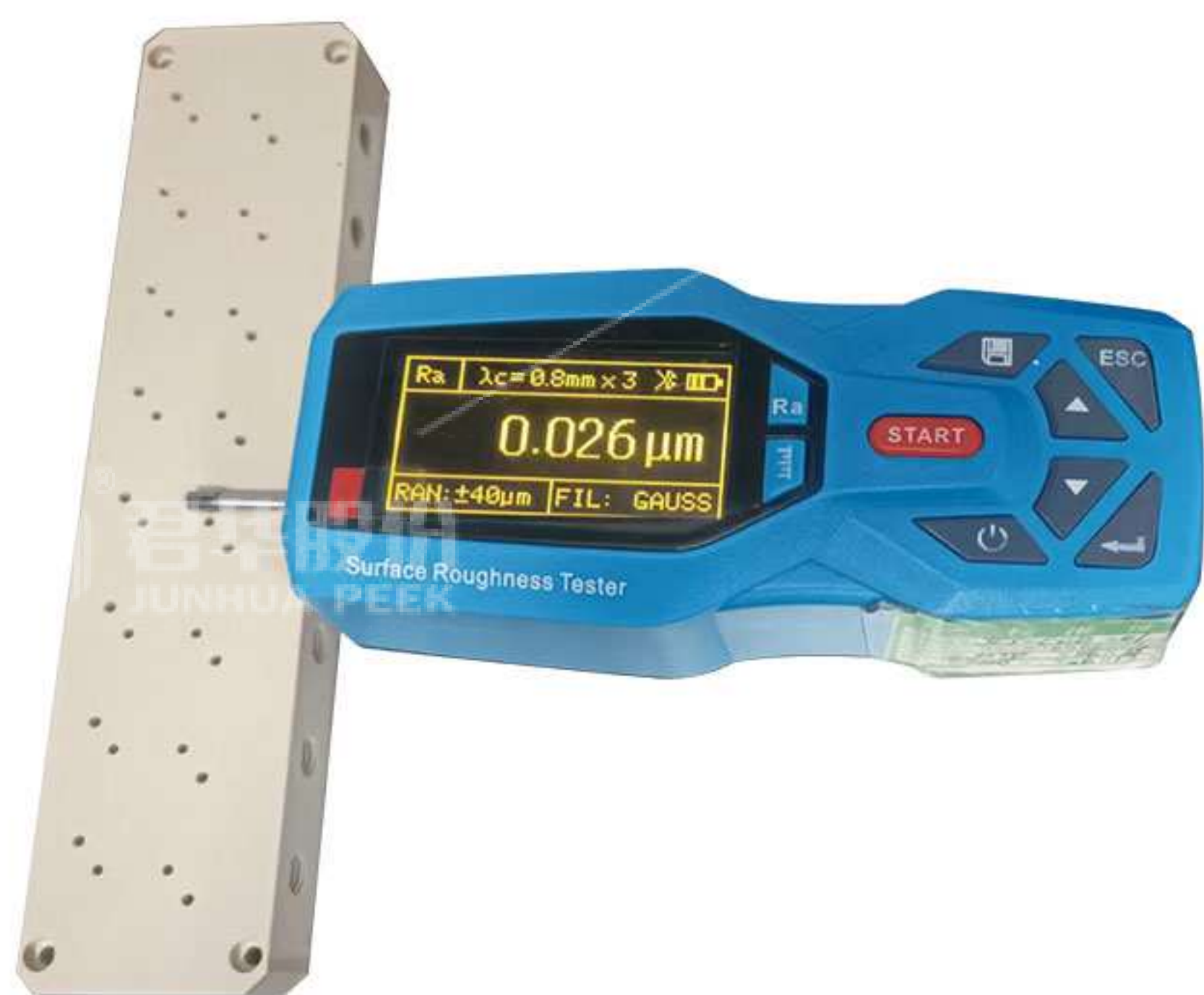
Test the surface roughness of valve base plate
