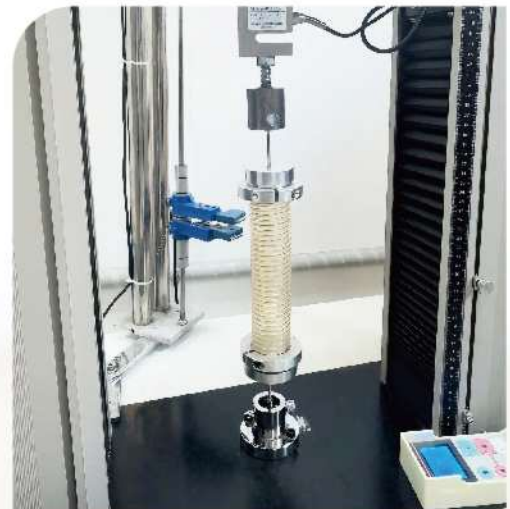
Tensile Performance Testing of Different PEEK Corrugated Tubing Samples
